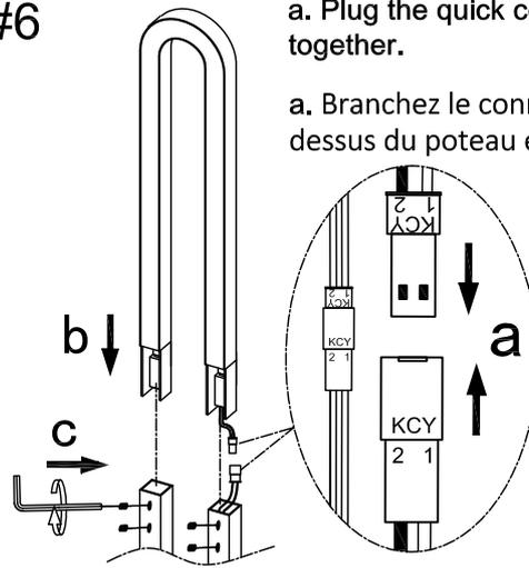
a. Plug the quick connector on top of pole together.
