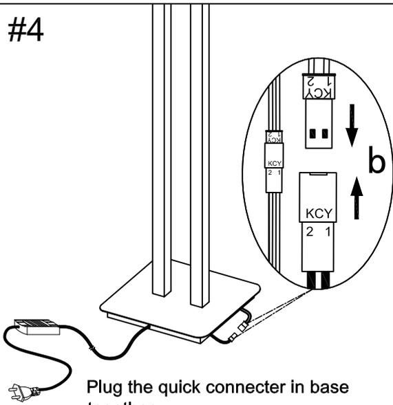
Plug the quick connector in base together.
