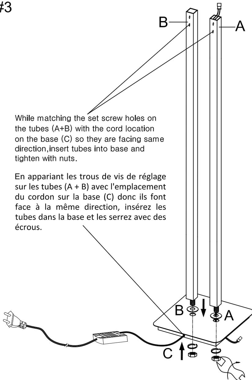
While matching the set screw holes on the tubes (A+B) with the cord location on the base (C) so they are facing same direction, insert tubes into base and tighten with nuts.
