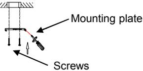
Attach the mounting plate to junction box with screws
