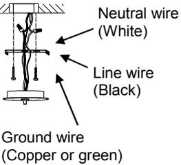
Connect the GROUND WIRE from junction box to GROUND (or GREEN) with from fixture by using a wire nut. (Or attach them to the mounting plate with a green ground screw) Connect the NEUTRAL WIRE from junction box to NEUTRAL (or WHITE) wire from fixture with a wire nut. Connect the LINE WIRE from junction box to LINE (or BLACK) wire from fixture with a wire nut.
