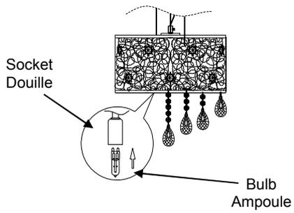
Insert the G9 bulb to the socket.
