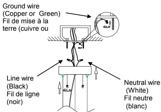
Connect the **GROUND WIRE** from junction box to **GROUND** (or **GREEN**) from fixture by using a wire nut. Connect the **NEUTRAL WIRE** from junction box to **NEUTRAL** (or **WHITE**) wire from fixture with a wire nut. Connect the **LINE WIRE** from junction box to **LINE** (or **BLACK**) wire from fixture with a wire nut.
