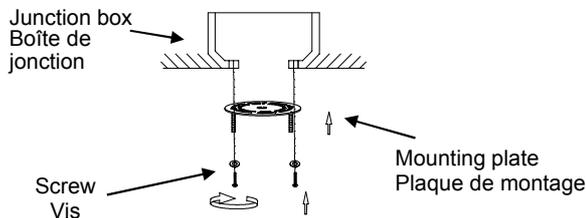
Attach the mounting plate to junction box with screws.
