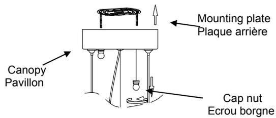
Install the canopy to mounting plate with cap nut provided.
