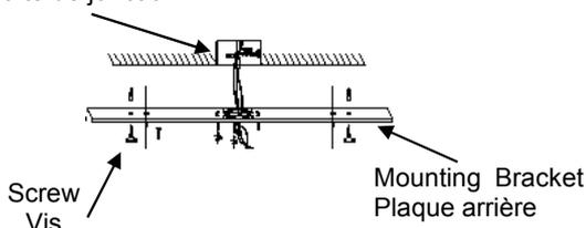
Attach the mounting plate to junction box with screws.
