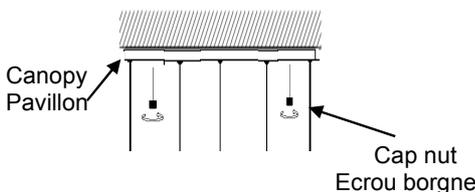
Install the canopy to mounting plate with cap nuts provided.
