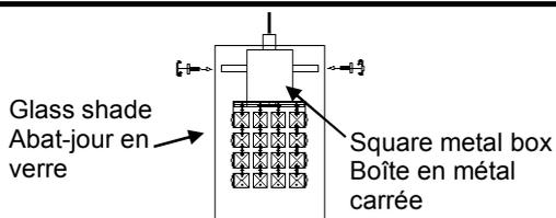
Install the glass shade to the lamp holder using screws provided. Do not over tighten!
