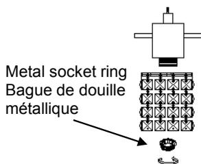
Install the square metal support bracket to the lampholder using the socket ring
