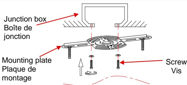
Attach the mounting plate to junction box with screws provided.
