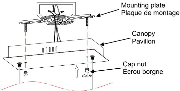
Install the canopy to mounting plate with 2 cap nuts provided.
