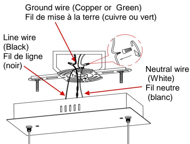
Connect the **GROUND WIRE** from junction box to **GROUND** (or **GREEN**) with from fixture by using a wire nut. (Or attach them to the mounting plate with a green ground screw)Connect the **NEUTRAL WIRE** from junction box to **NEUTRAL** (or **WHITE**) wire from fixture with a wire nut.Connect the **LINE WIRE** from junction box to **LINE** (or **BLACK**) wire from fixture with a wire nut.
