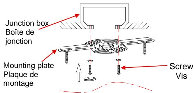
Attach the mounting plate to junction box with screws provided.
