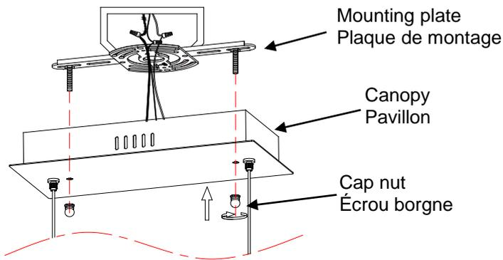
Install the canopy to mounting plate with 2 cap nuts provided.
