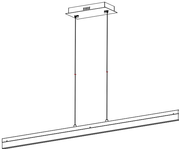
This fixture is designed to dim with a standard Triac forward phase dimmer. Dimming levels will vary by dimmer.
