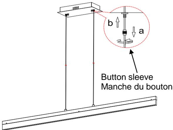
Before installation to ceiling, adjust fixtures to desired length by pushing wire up into canopy, then coiling up excess wire, minor adjustment can be made after installation. To lower or lengthen wire, depress button sleeve located where wire comes out of canopy.
