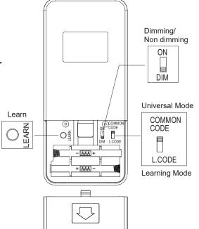
Remote Control Fan Speed And Light Functions.
