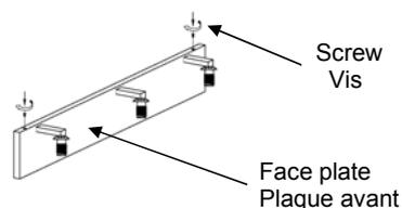
Attach the face plate to the back plate with screws provided.
