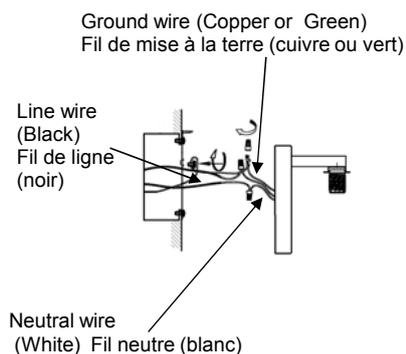
Connect the GROUND WIRE from junction box to GROUND (or GREEN) with a wire nut. Connect the NEUTRAL WIRE from junction box to NEUTRAL (WHITE) wire from fixture with a wire nut. Connect the LINE WIRE from junction box to LINE (BLACK) wire from fixture with a wire nut.
