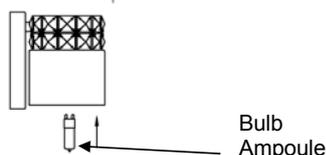
Insert the G9 bulb to the socket.
