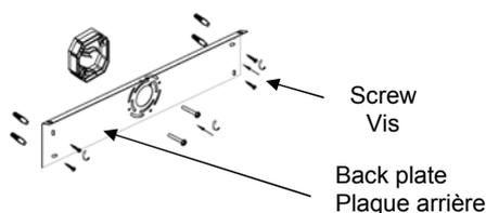
Attach the back plate to the junction box.
