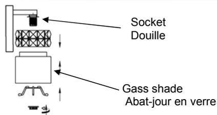
Install the glass shade on the lampholder, Do not over tighten.
