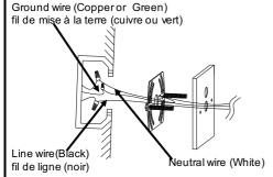
Connect the GROUND WIRE from junction box to GROUND (or GREEN) with a wire nut. Connect the NEUTRAL WIRE from junction box to NEUTRAL (WHITE) wire from fixture with a wire nut.Connect the LINE WIRE from junction box to LINE (BLACK) wire from fixture with a wire nut.
