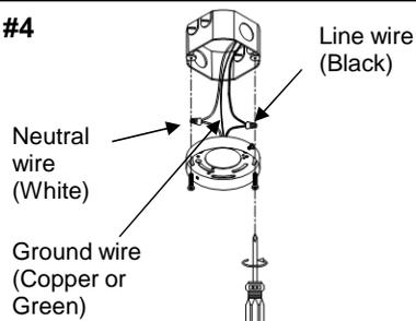
Connect the GROUND WIRE(Green or Copper) from junction box to GROUND WIRE(Labeled) from fixture by using a wire nut. Connect the NEUTRAL WIRE(White wire) from junction box to NEUTRAL WIRE(Labeled) from fixture with a wire nut. Connect the LINE WIRE(Black wire) from junction box to LINE WIRE(Labeled) from fixture with a wire nut
