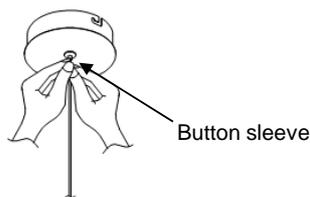
Before installation to ceiling, adjust fixtures to desired length by pushing wire up into canopy, then coiling up excess wire, minor adjustment can be made after installation. To lower or lengthen wire, depress button sleeve located where wire comes out of canopy.
