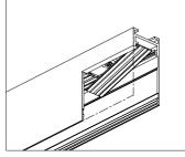
STEP 6 SLIDE MSAS03 TRACK CORNER ONTO THE TRACK CONNECTOR (a) WHILE CAREFULLY LINING UP THE PIN SET ON THE TRACK WITH THE PIN SET HOLES ON THE TRACK CORNER.
