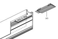
STEP 5 INSTALL THE MSA22 PIN SET(b) INTO THE PIN CONNECTOR HOLES (c) ON THE TRACK. SLIDE THE TRACK CONNECTOR (a) INTO THE SLOT ON THE BACK OF THE TRACK APPROXIMATELY HALFWAY AND SECURE TO TRACK WITH TWO SET SCREWS.
