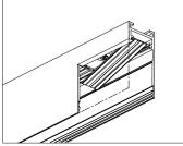
STEP 6 SLIDE MSAS06 TRACK CORNER ONTO THE TRACK CONNECTOR (a) WHILE CAREFULLY LINING UP THE PIN SET WITH THE PIN SET HOLES ON THE MSAS06 TRACK CORNER.
