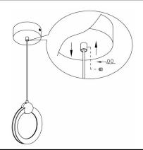
Before installation to ceiling, adjust fixtures to desired length by pushing wire up into canopy, then coiling up excess wire, minor adjustment can be made after installation. To lower or lengthen wire, loosen the screw where wire comes out of canopy.
