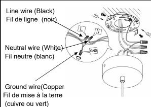
Connect the GROUND WIRE from junction box to GROUND (or GREEN) with a wire nut. Connect the NEUTRAL WIRE from junction box to NEUTRAL (WHITE) wire from fixture with a wire nut. Connect the LINE WIRE from junction box to LINE (BLACK) wire from fixture with a wire nut.
