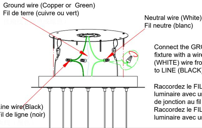
Connect the GROUND WIRE from junction box to GROUND (or GREEN) wire from fixture with a wire nut. Connect the NEUTRAL WIRE from junction box to NEUTRAL (WHITE) wire from fixture with a wire nut. Connect the LINE WIRE from junction box to LINE (BLACK) wire from fixture with a wire nut.
