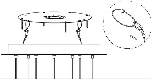
Attach the hooks on the fixture to the safety cable rings in the mounting plate to help hold the fixture while making the wiring connections.
