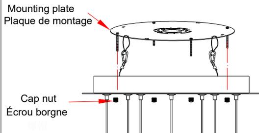
Install the canopy to mounting plate with cap nuts provided.
