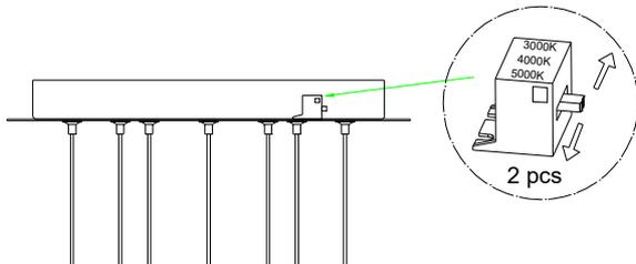
This fixture is a 3CCT selectable model. Default color temperature is 3000K. You can shift to 4000K or 5000K by sliding the the switch.
