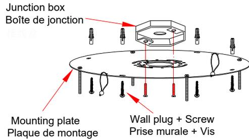
Attach the mounting plate to the junction box and ceiling with the wall plugs and screws provided.
