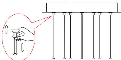
Before installation to ceiling, adjust fixtures to desired length by pushing wire up into canopy, then coiling up excess wire, minor adjustment can be made after installation. To lower or lengthen wire, depress button sleeve located where wire comes out of canopy.
