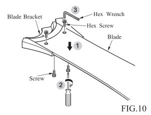
2. Attached each blade assembly to the fan body using the blade bracket screws. Tighten them securely. (See fig.11)
