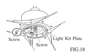
3. Remove 1 of 3 screws on light kit plate, and loosen the other 2 screws.(See fig.19)
