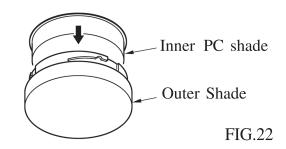
7. Attach the outer shade by locating tabs in light kit with grooves on the light shade and twist clockwise until tight. (See fig.23)
