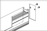
STEP 2 INSTALL THE MSA22 PIN SET(b) INTO THE PIN CONNECTOR HOLES (c) ON THE TRACK. SLIDE THE TRACK CONNECTOR (a) INTO THE SLOT ON THE BACK OF THE TRACK APPROXIMATELY HALFWAY AND SECURE TO TRACK WITH TWO SET SCREWS.
