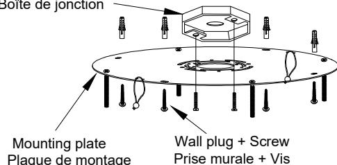
Attach mounting plate to junction box and ceiling with the wall plugs and screws provided.
