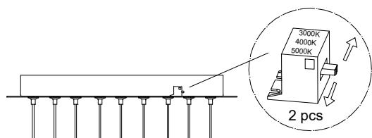
This fixture is a 3CCT selectable model. Default color temperature is 3000K. You can shift to 4000K or 5000K by sliding the switch.
