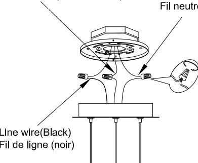
Connect the GROUND WIRE from junction box to GROUND (or GREEN) wire from fixture with a wire nut. Connect the NEUTRAL WIRE from junction box to NEUTRAL (WHITE) wire from fixture with a wire nut. Connect the LINE WIRE from junction box to LINE (BLACK) wire from fixture with a wire nut.
