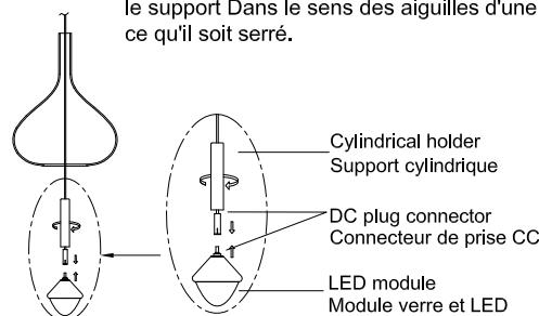
4. Gently slide the glass downward onto the LED module.
