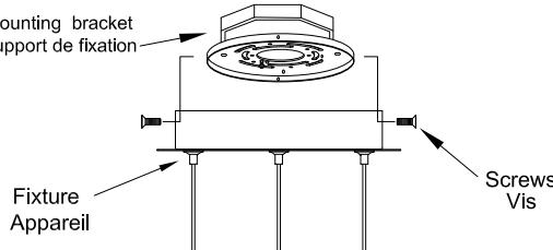
Attach the fixture to the mounting plate with screws provided.
