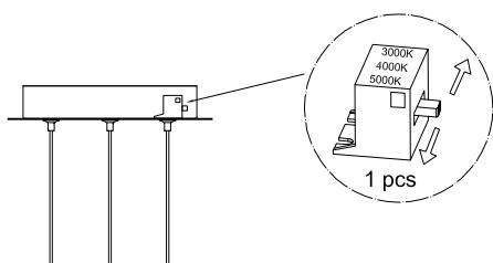
This fixture is a 3CCT selectable model. Default color temperature is 3000K. You can shift to 4000K or 5000K by sliding the the switch.
