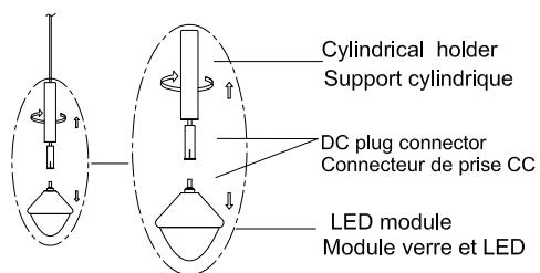
2. Insert the glass upward through the cylindrical holder.
