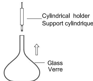
3. Plug the DC connector. Slide the cylindrical holder down and secure the LED module by twisting the holder clockwise until tight.
