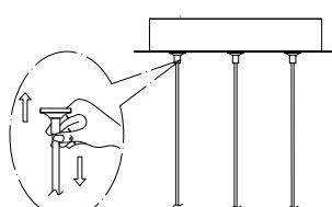
Before installation to ceiling, adjust fixtures to desired length by pushing wire up into canopy, then coiling up excess wire, minor adjustment can be made after installation. To lower of lengthen wire, depress button sleeve located where wire comes out of canopy.
