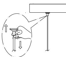
Before installation to ceiling, adjust fixtures to desired length by pushing wire up into canopy, then coiling up excess wire, minor adjustment can be made after installation. To lower of lengthen wire, depress button sleeve located where wire comes out of canopy.
