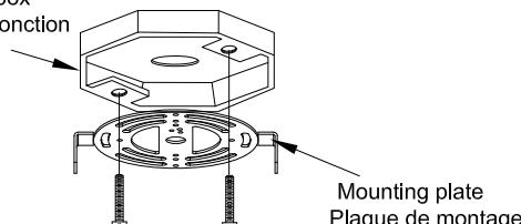
Attach the mounting plate to junction box with screws provided.
