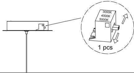
This fixture is a 3CCT selectable model. Default color temperature is 3000K. You can shift to 4000K or 5000K by sliding the the switch.
