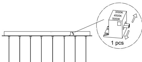
This fixture is a 3CCT selectable model. Default color temperature is 3000K. You can shift to 4000K or 5000K by sliding the the switch.
